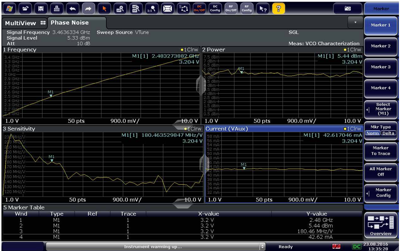
Fig. 2: A typical VCO measurement. Key parameters such as frequency, power, sensitivity (tuning slope) and current consumption are measured relative to the tuning voltage.
