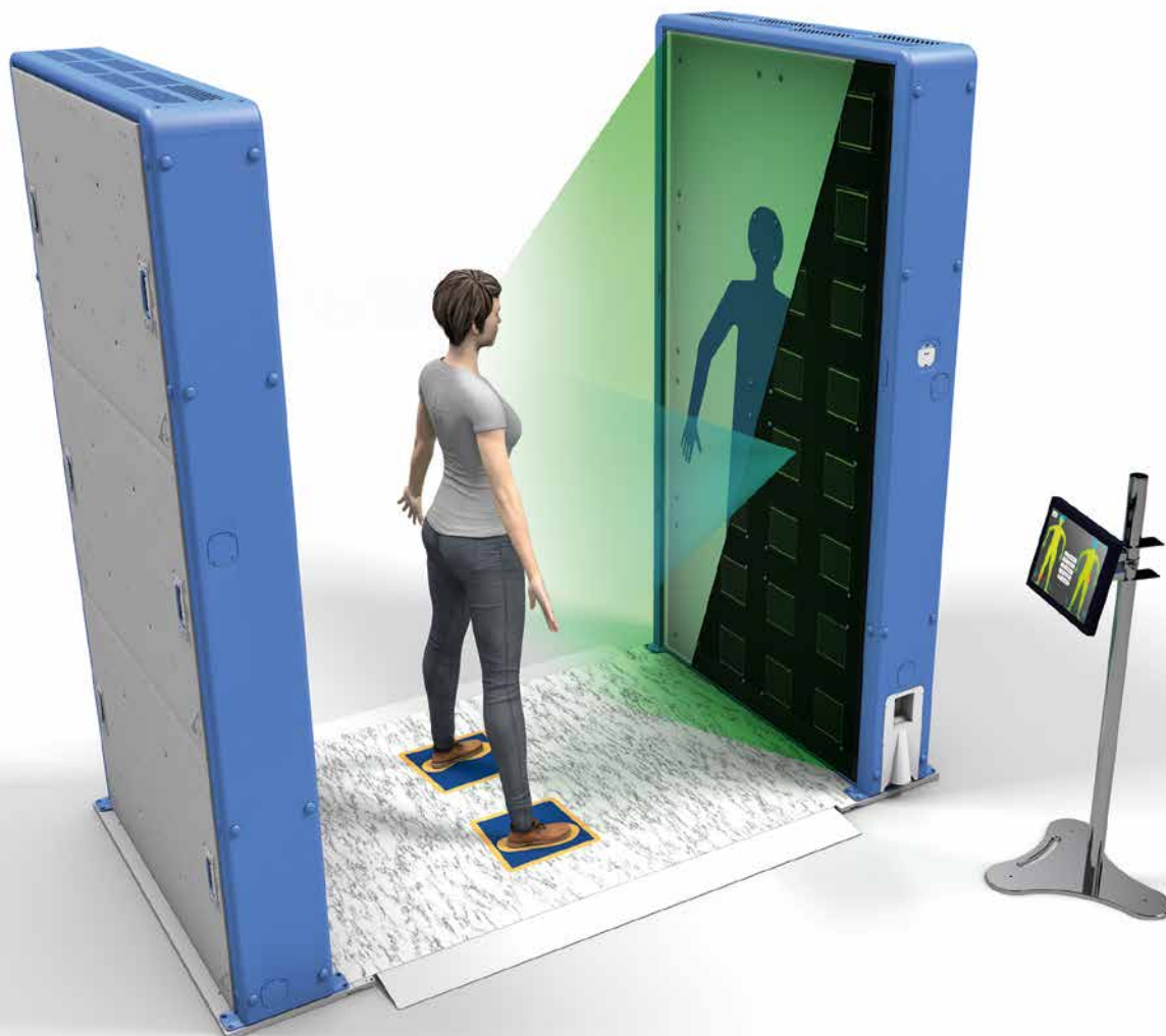
Fig. 3: Multistatic principle of operation: While only one of the 3008 transmitters is active at a time in a panel, all 3008 receiving antennas receive the reflected signal. Since every transmitter also rapidly steps through 128 frequencies before the next one starts transmitting, each scan cycle delivers more than a billion (!) complex values per panel (magnitude and phase), all within only 32 ms.
