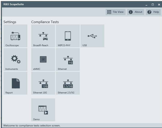
Fig. 7: The main screen of the R&S®ScopeSuite shows the available compliance tests.
