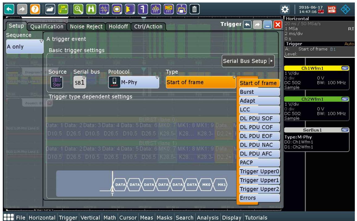
Fig. 11: M-PHY® / UniPro protocol decoding setup.
